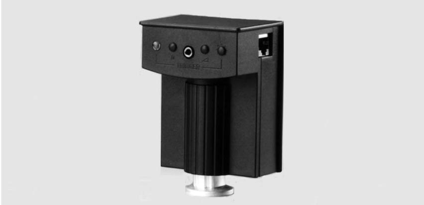
The THERMOVAC transmitters have been developed especially for integration into vacuum systems. Being active sensors (pressure to voltage converters) with a well-proven Pirani sensing cell and new operating and processing electronics these units offer a measurement range which spans  $5 \times 10^{-4}$  to 1000 mbar ( $3.75 \times 10^{-4}$  to 750 Torr).
