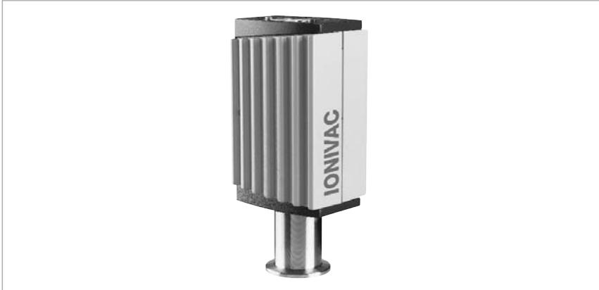
The ITR 90 is an optimized combination transmitter. The combination of a hot cathode ionisation sensor according to Bayard-Alpert and a Pirani sensor permits vacuum pressure measurements of nonignitable gases and gas mixtures in the pressure range from  $5 \times 10^{-10}$  to 1000 mbar.
