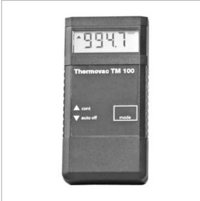
The handheld THERMOVAC TM 100 is capable of measuring pressures within the pressure range of 1200 to  $5 \times 10^{-4}$  mbar (900 to  $3.75 \times 10^{-4}$  Torr). By combining a piezo-resistive pressure sensor for the upper and a Pirani sensor for the lower pressure range, the measurements made by the THERMOVAC TM 100 are independent of the type of gas above pressures of 15 mbar. Especially noteworthy is the exceptionally long battery life.
