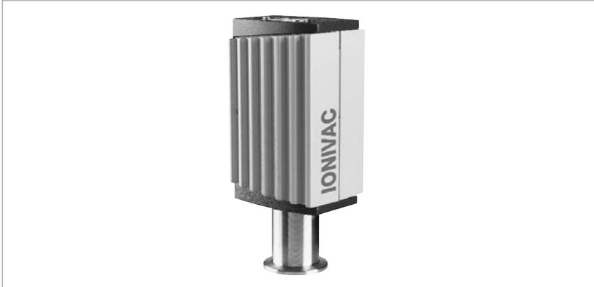
The ITR 200 S is an optimised dual cathode combination transmitter on the basis of the well proven ITR 90. The combination of a hot cathode ionization sensor according to Bayard-Alpert and a Pirani sensor allows vacuum pressure measurements of non-ignitable gases and gas mixtures in the pressure range from  $5 \times 10^{-10}$  to 1000 mbar.
