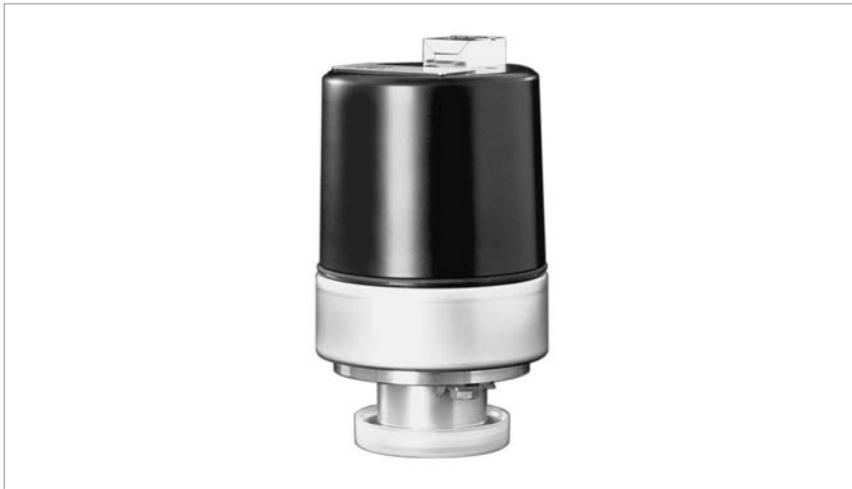
The PENNINGVAC transmitter combines the cold cathode ionization principle with the Pirani principle. This allows for complete coverage of the pressure range from  $5 \times 10^{-9}$  mbar to atmospheric pressure by a single transmitter. The cold cathode system is ignited directly through switching on the internal high-voltage at the optimum ignition pressure.
