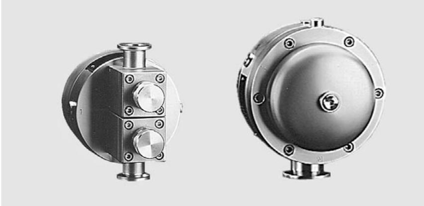
The MR 16/50 diaphragm regulators are absolute pressure regulators which automatically adapt the pumping speed of a vacuum pump depending on the amount of gas, without the need for an external power supply.
