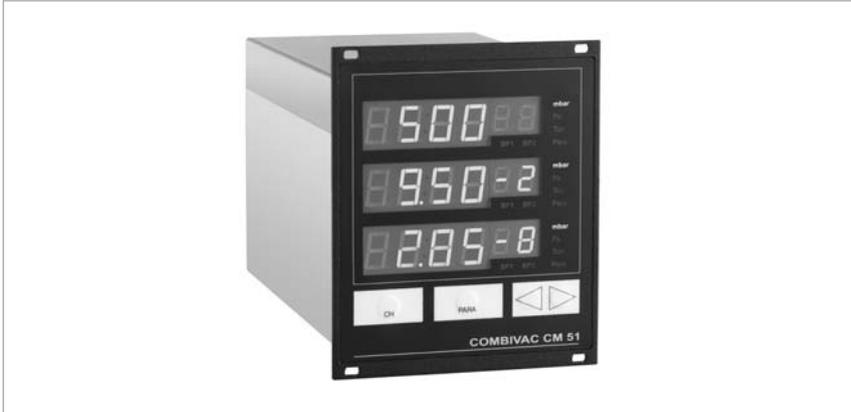
The COMBIVAC CM 51 covers the complete pressure range between  $10^{-9}$  and 1000 mbar by combining two measurement principles - THERMOVAC and PENNINGVAC - providing both monitoring and control functions.
