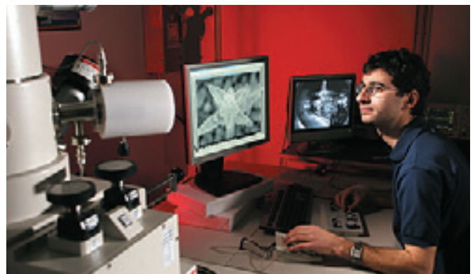
Scanning electron microscopes, like the one shown here, can "see" details as small as one nanometre – one millionth of a metre!
